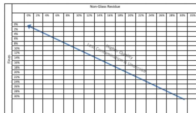
Since there are many different generations of Material Recovery Facilities (MRFs), cleaning equipment in operation, and curbside collection programs, the quality generated by MRFs varies widely. Processors evaluate this heterogeneous material by evaluating the amount of:
